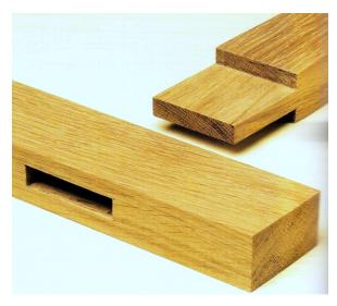
Fig 3.1.6.1: Mortise and Tenon Joint
