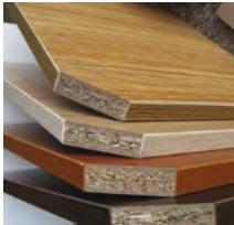
Fig 3.2.1.8: Samples of particle board (chipboard)
