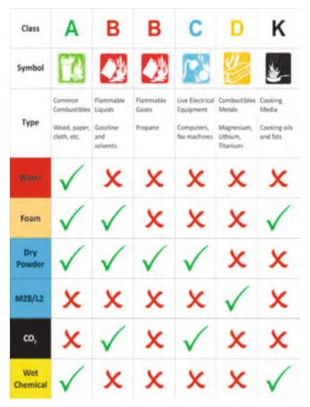
Fig 12.1.3.1: Fire Extinguishing Code
